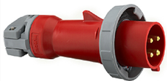
Watertight IEC Pin and Sleeve Plug, 4P5W, 30A 3PH 277/480V
