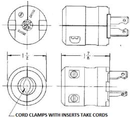
FROM 19/64 TO 29/64 DIA. & WITHOUT INSERTS FROM 29/64 TO 11/16 DIA.
